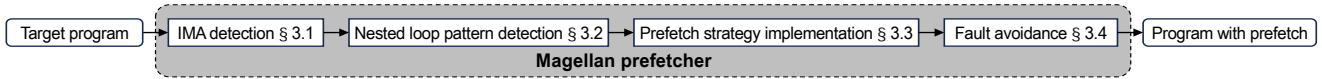
Figure 6: Magellan takes four steps to insert efficient and safe prefetching instructions for a target program.
